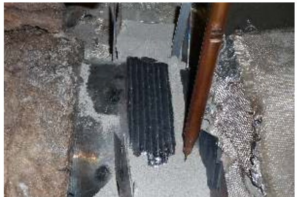
Gebrochene Welle D=450mm 34CrNiMo6
