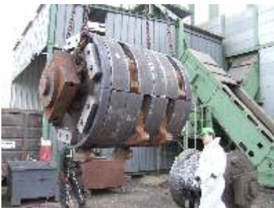
Assembly of Rotors with new protective Caps
