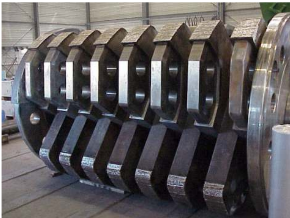
Rotor for assembling with protective caps Free surfaces protected by hard welding
