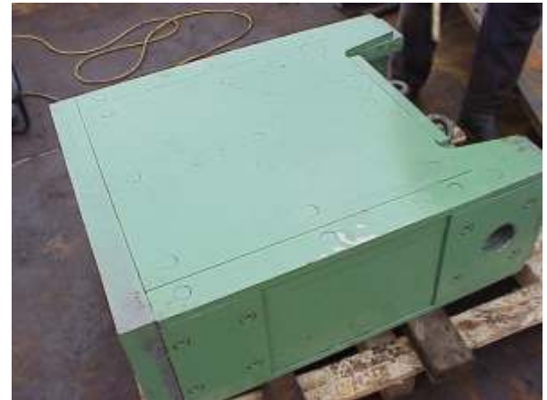
Tamper after repair
