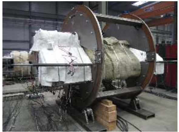
Facilitating of welding using Rhönrad
