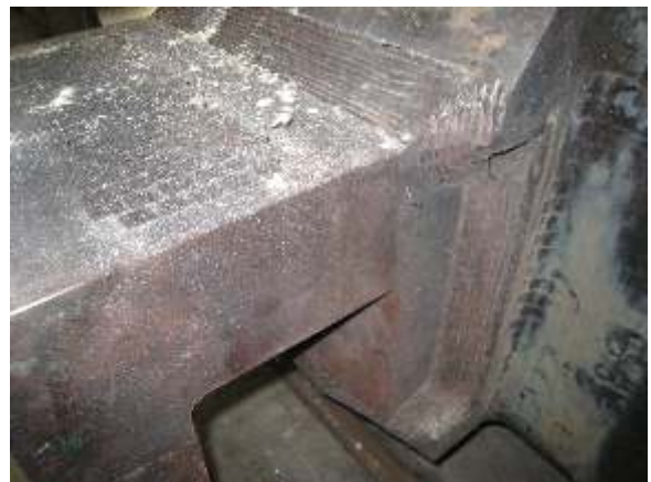
Welded coupling part from 25CrMo4
