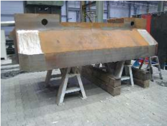
Workpiece before the welding process GS 25 CRNiMo 4
