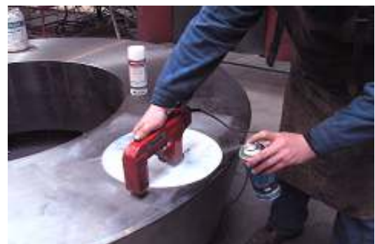
Magnetic powder testing of a stamping ring
