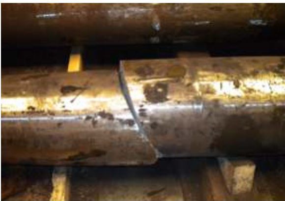
Broken Shaft Diameter 450mm
