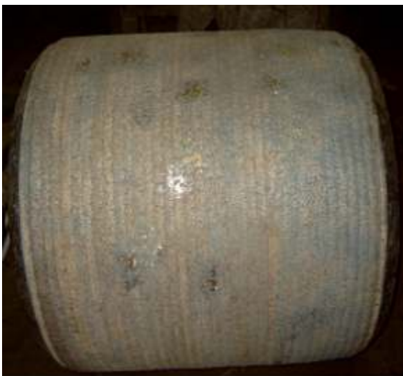
Roll Barrel Material 18 NiCrMo 14 6 Hard Coating built-up welding 56 - 58 HRc
