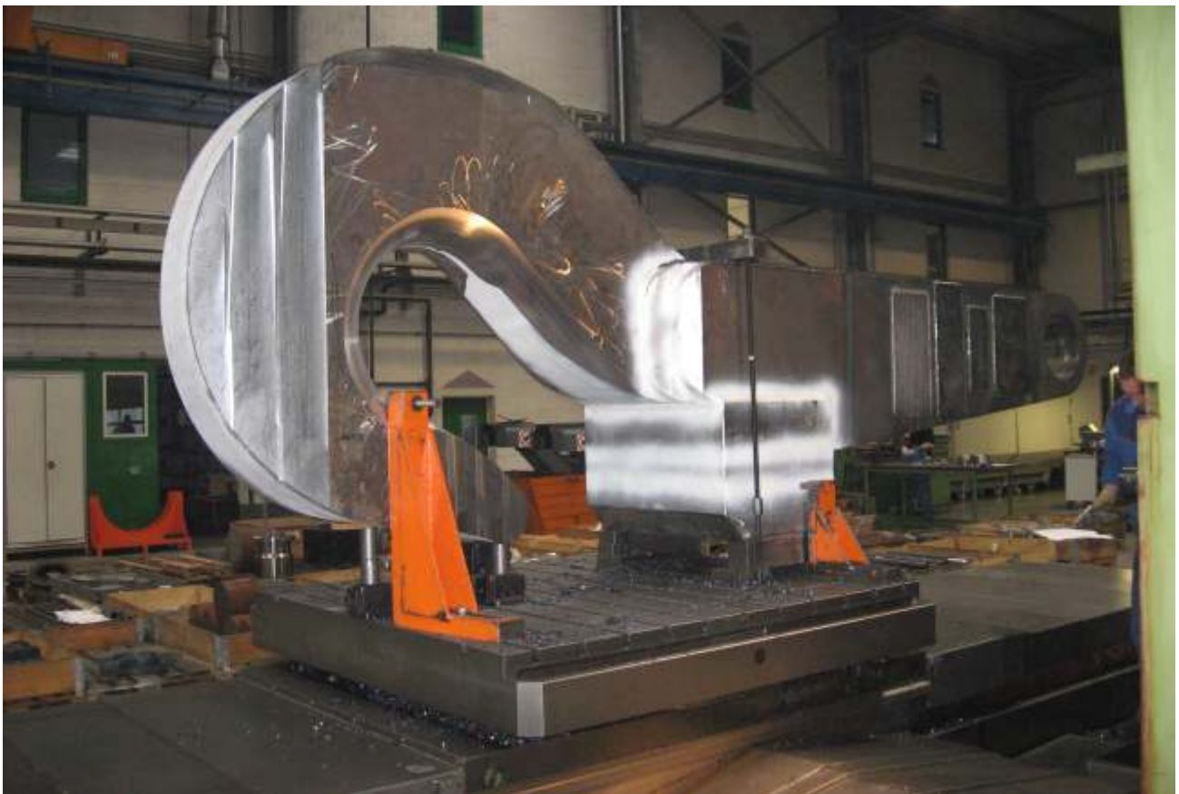
Machining operation of a hoak, load capacity 200t
