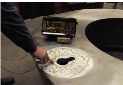
Ultrasonic testing of a stamping ring
