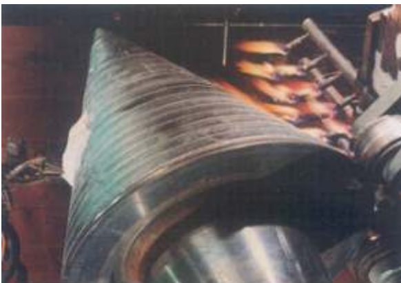
Axial Ring Roller Material 56 NiCrMo V
