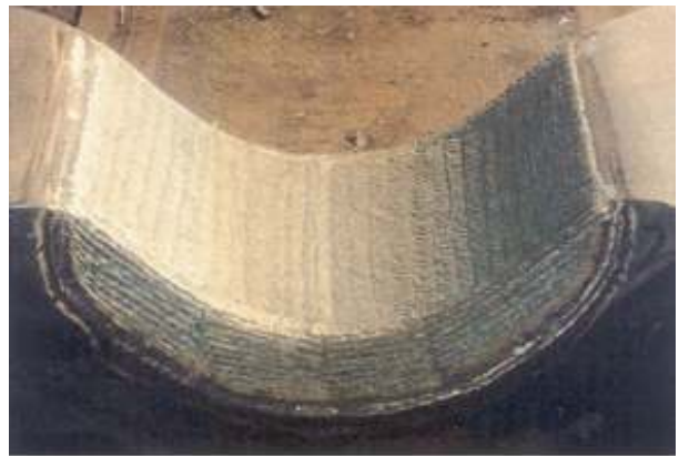
Forging saddle Material 56 NiCrMo V
