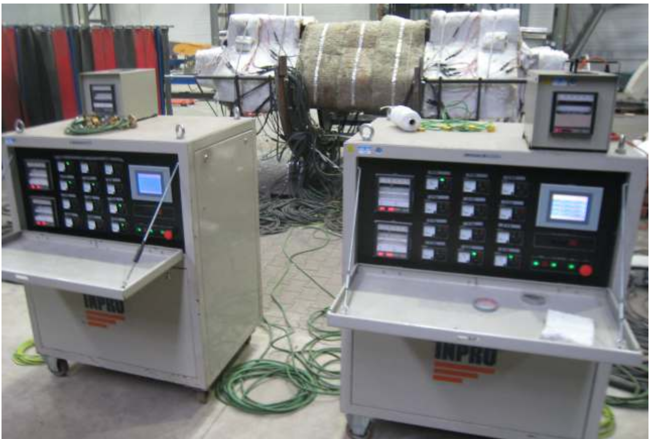
Heating Devices with 12 temperature control circuits Equipment performance: 84KVA / unit
